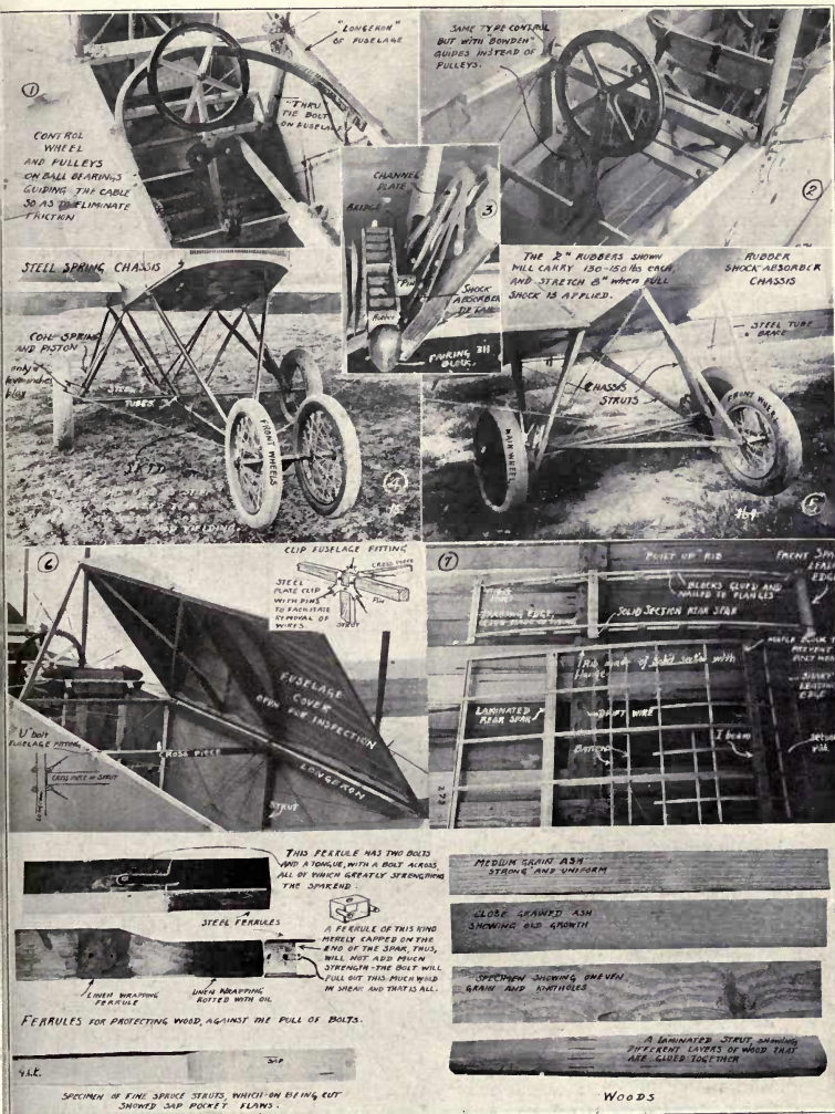
1. Control with cables and pulleys on ball bearings. — 2. Same with friction leads. — 3. Detail of rubber shock absorber bridge. — 4. Steel Spring chassis, with central skid. — 5. Softer rubber chassis with no skid. Both of them are typical chassis for exactly the same work. — 6. Fuselage details. — 7. Details of wing frames, ferrules and lumber.
